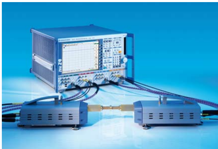
Setup for a two-port measurement showing a through connection. A four-port network analyzer eliminates the need for controlling an external generator that supplies the LO signals.
